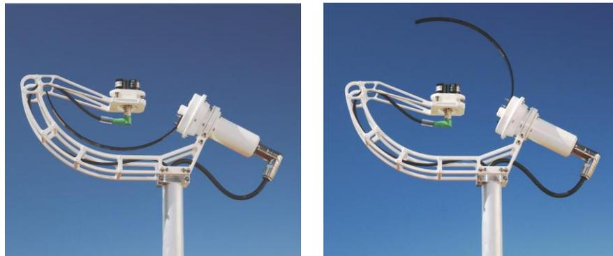
***CSP Services Twin-Sensor Rotating Shadowband Irradiometer (RSI)
