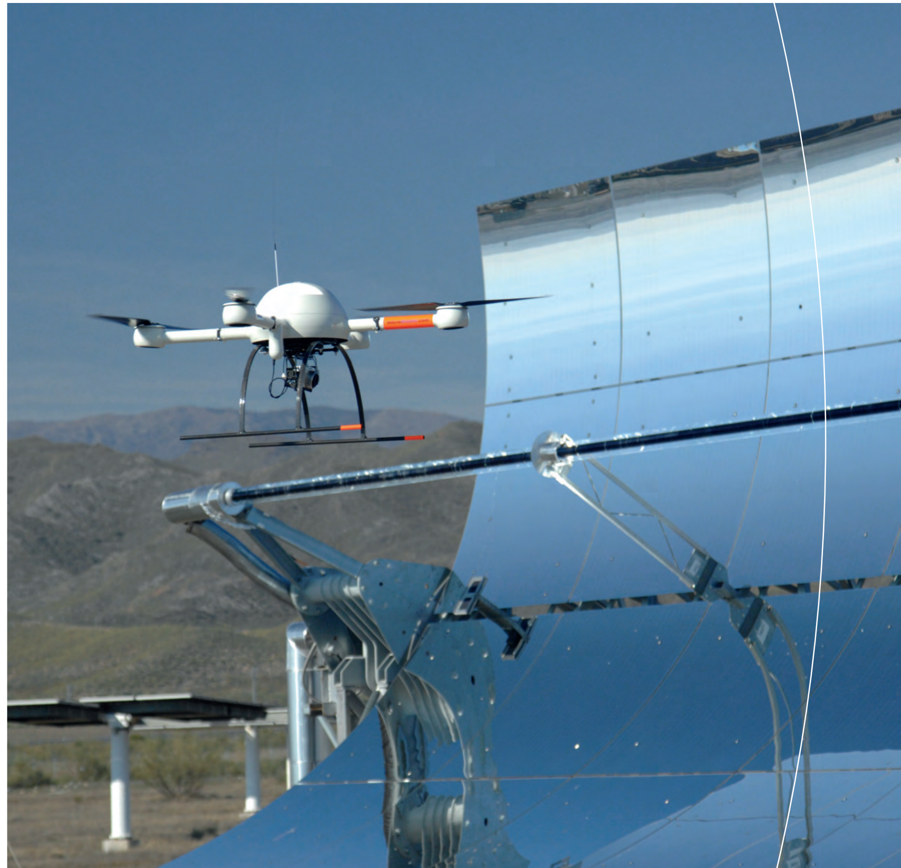
Fast data acquisition from the air. The parabolic mirrors of a solar power plant are measured using the flying camera system QFly. With the data, operations can be optimised and the yield can be increased.
