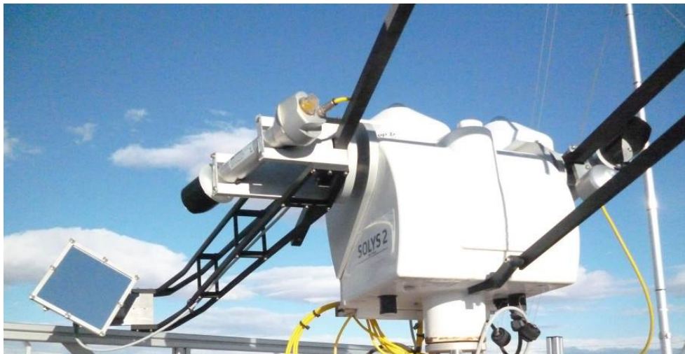
TraCS instrument installed on Kipp & Zonen sun tracker Solys 2
