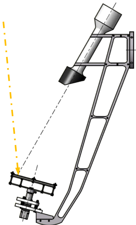
TraCS setup with pyrheliometer, mirror and drive
