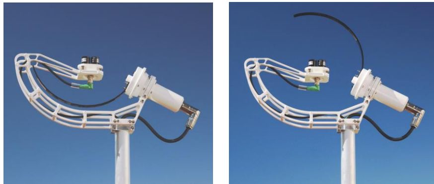
CSP Services Twin-Sensor Rotating Shadowband Irradiometer (RSI) in rest position (left) and during the rotation (right)
